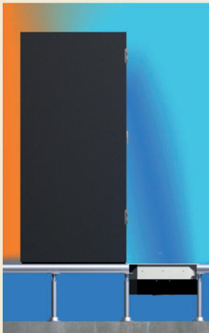
A mean is calculated from the two temperature sensors and compared with the controller setpoint. If the temperature difference between the mean and setpoint increases, the dampers open, increasing the flow of cool air from the raised floor to the servers.
