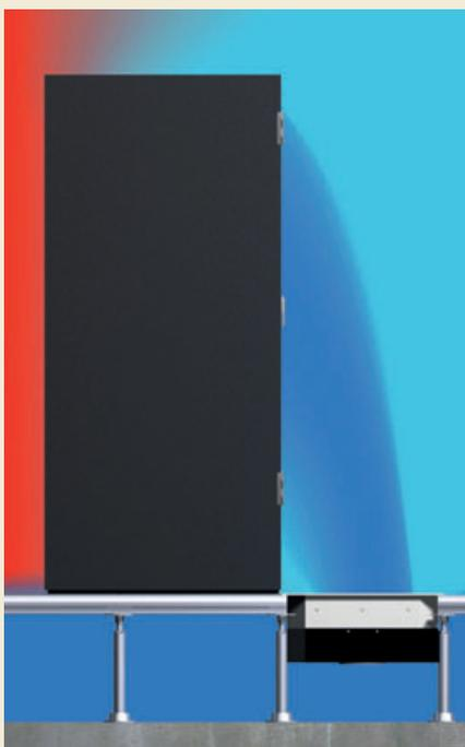
If the temperature difference between the mean and setpoint increases, the EC fan speed increases correspondingly
